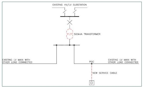
300kVA transformer at the local substation with a 500kVA transformer.
