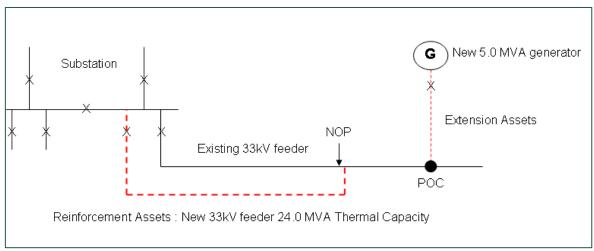
diagram below, rather than upgrade the existing 33kV feeder to the same point along it
