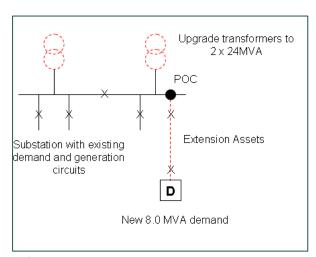
includes the Customer) to comply with the requirements of Engineering Recommendation P2/6. As the Extension Assets will be provided solely for the Customer, these can be provided on the basis of a single circuit to provide a non-secure connection, at the Customer's request.
