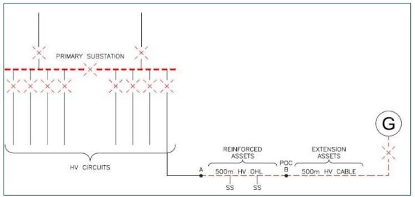
substation in order to increase its fault level rating from 150MVA to 350MVA. However, the new fault level will be limited by the fault level rating of the local network of 250MVA.
