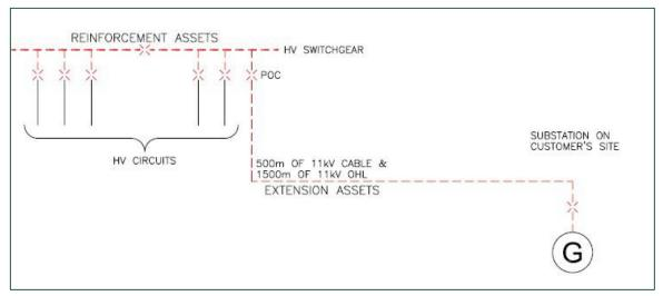
the generator necessitates Reinforcement works to replace the 11kV switchgear at the existing primary substation with switchgear of a higher fault level rating.
